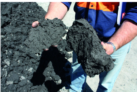
Dry cake ready to be transported to deposit
