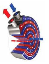
A spiral heat exchanger is circular with two concentric spiral channels, one for each fluid. The curving channels provide extremely efficient heat transfer.
