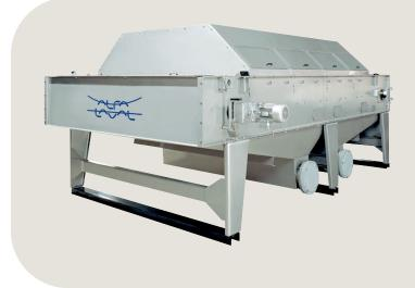
flocculated sludge rises up over a weir to ensure even distribution onto the belt. Sludge ploughs force the sludge into lanes which allows free water to run through the filter belt where sludge is not present, thus enhancing the thickening process. The ramp allows the thickened solids content of the product to be precisely adjusted and fine tuned during operation.
